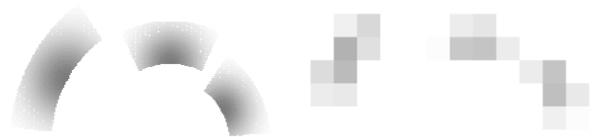
Figure 2. Sensor data shown on both a high-granularity [1cm resolution], sensor model (left) and then the same data on low-granularity [25cm resolution] (right) sensor plane. Dark colours represent a high probability of obstacles, whereas light colours represent a lower probability. White areas indicate where there are no obstacles.
